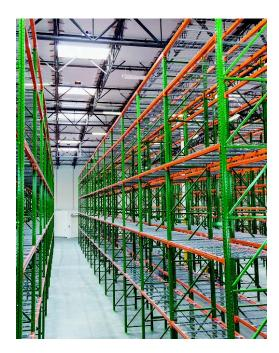
Know your environment and know your products as you plan what kind of racking to install. A tougher environment (outdoor, freezer, and cooler) with heavier materials calls for structural racking since it can withstand more abuse. Roll formed pallet racking is tough enough for most warehousing environments and it's typically a very cost-effective option.
